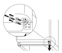
3. Remove the door fitting from the door bearing (1, 2). Move the bearing pivot from the right to the left hand hole (3). Place the door fitting supplied on the bearing pivot (4, 5).
